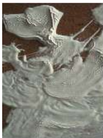
Image 5. The mixture of lead white and sun-thickened linseed oil (shown on Image 4) two weeks after application.
