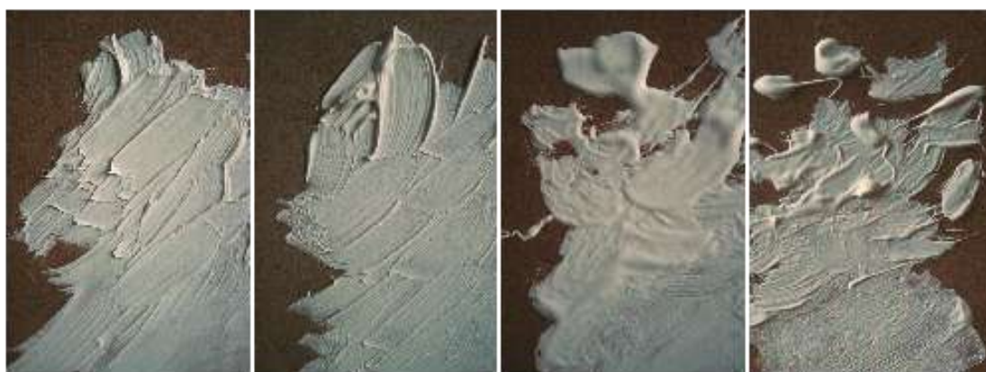
Image 4. Lead white painting experiment. From left to right: linseed oil; black oil; sun-thickened linseed oil; sun-thickened linseed oil with egg yolk.
